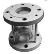
Sight glass is a device used to check inline flow of liquids in Horizontal as well as Vertical Installations. It enables maintaining flow of the liquid by viewing instaneously and guides for any subsequent change in flow desired.
